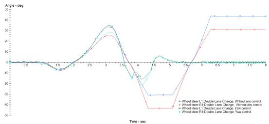
Fig.10 The front wheel steering Angle curve
