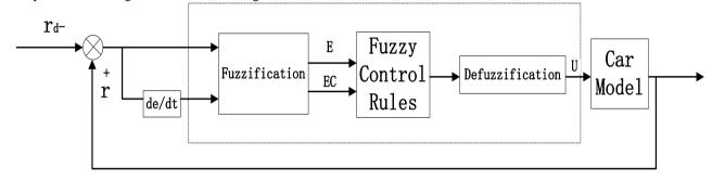
Fig.3 fuzzy controller system block diagram
