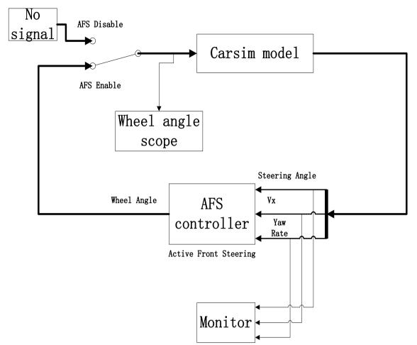
Fig.1 architecture description diagram
