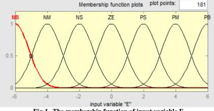
Fig.4 The membership function of input variable E
